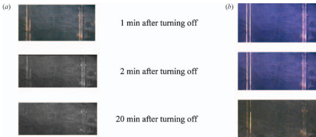
Figure 6. Images of a cell after turning off electric field; PA treatment, wedge-like cell, d \approx 30 \mu\text{m} , g = 100 \mu\text{m} , J = 0.2 \text{ J cm}^{-2} : (a) excitation time t_{\text{ex}} = 35 \text{ min} ; (b) t_{\text{ex}} = 65 \text{ min} .
